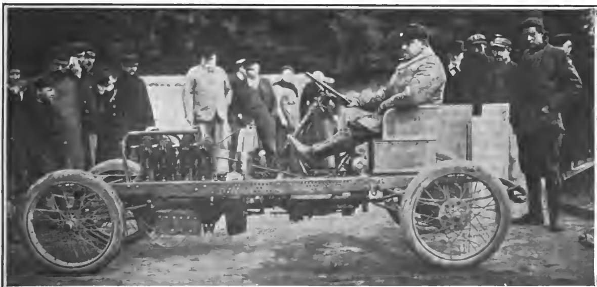
FIG. 1.—VULPES AIR-COOLED 18-24-HORSEPOWER SPECIAL SPRINT RACER, WITH WHICH BARRIAUX BROKE THE KILOMETER RECORD FOR CARS WEIGHING 900 POUNDS.
